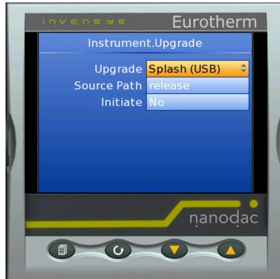
Splash screens are prepared by the user and transferred using a memory stick. The unit restarts automatically after an upgrade or splash screen replacement.
